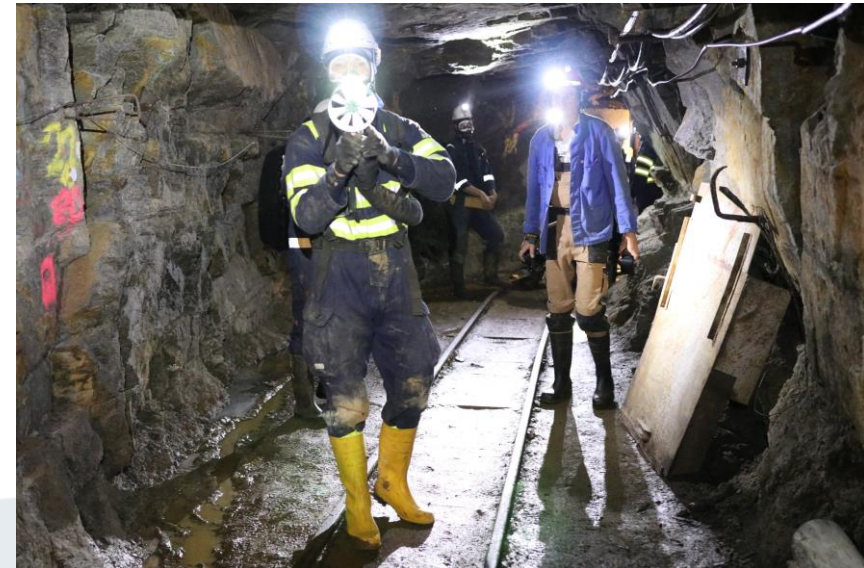
Ventilation measurements underground (Source: Dalibor Kuhinek)
